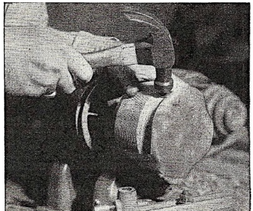
After the cup is turned the sheet to be turned is tacked on stoutly in at least four places. It is better to leave ears on the metal and turn them down this way.
