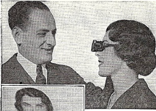
Above photo shows how the new telescopic lens for the near-blind is worn. The lens is a set of three cylindrical lenses set in a compact frame an inch thick, and brings almost normal vision to eyes with as little as two per cent sight. Magnification is in a horizontal direction only, making object appear wider but not bringing them closer, as may be seen in the photo at the left, which is a view the wearer of the lens gets.
